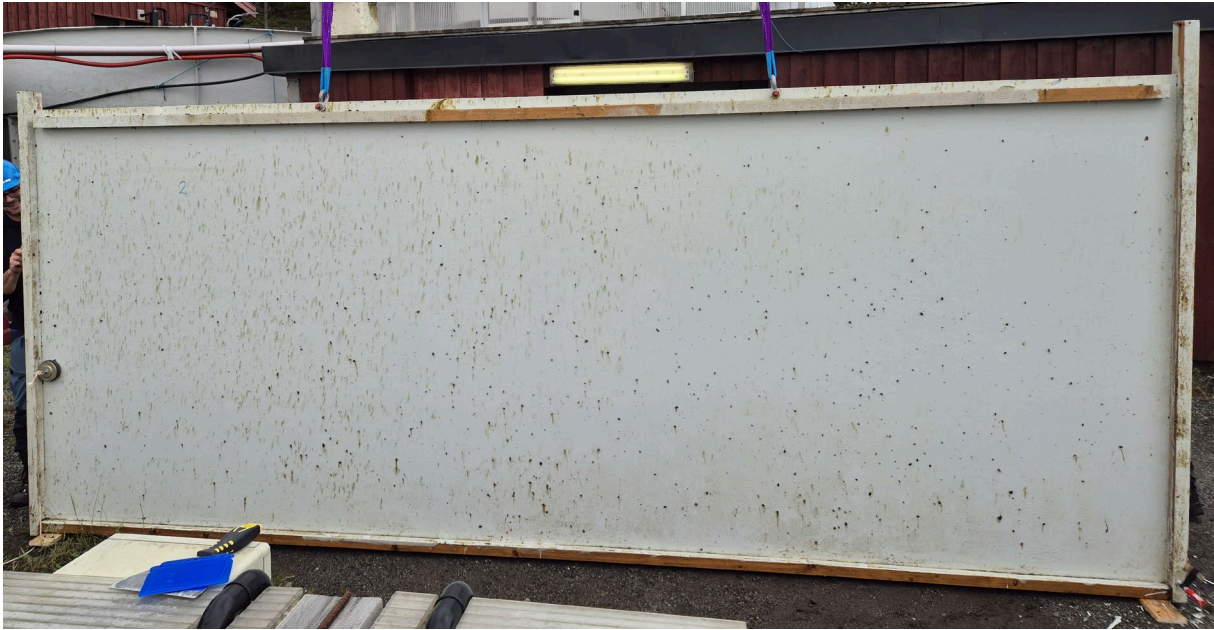
Figure 2-2. Picture of Plate 1 prior to treatment in WST2. Macro biofilm (visible green and brownish threads and spots) covers 20-30 % of surface. There were 50-100 blue mussels per plate. The macrofouling coverage was estimated to be >1% of the plate's surface, i.e. biofouling rating "2" according to IMO. Source NIVA.
